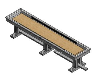
4 INSTALL THE STRETCHERS BY SLIDING THEM THROUGH THE CENTER OF THE LEGS TOWARD THE CENTER OF THE TABLE. THEY SIMPLE REST IN PLACE ON TOP OF PRE-INSTALLED BLOCKS ON THE LEGS. VELCRO STRAPS KEEP THE STRETCHER IN PLACE. NO HARDWARE IS REQUIRED.
