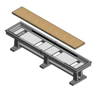
5 SET TWO SHUFFLEBOARD PUCKS ON EITHER END OF THE TABLE, THEN GET HELP TO LIFT THE PLAYFIELD INTO THE CRADLE, ON TOP OF THE PUCKS. FROM UNDERNEATH THE TABLE, LIFT THE PLAYFIELD AND REMOVE THE PUCKS. LEVEL THE TABLE USING THE ADJUSTABLE LEVELS ON THE LEG.
